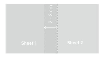
Concerning the overlapping application with twinseam cut apply two sheets of films overlapping (approx. 2-3 cm).
