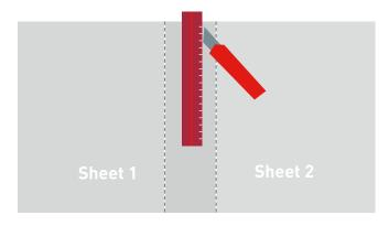
Afterwards cut both sheets approximately in the middle of the overlap using cutter and ruler.
